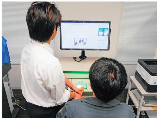
**live scanners that can collect the fingerprints of suspects**
